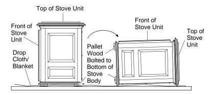
Figure 7 - Laying Down Stove On Side
